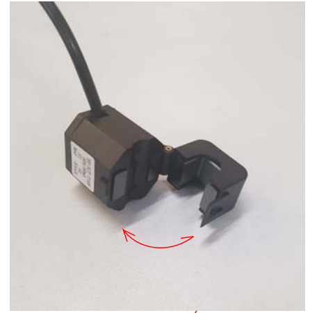
Transformer opening direction
